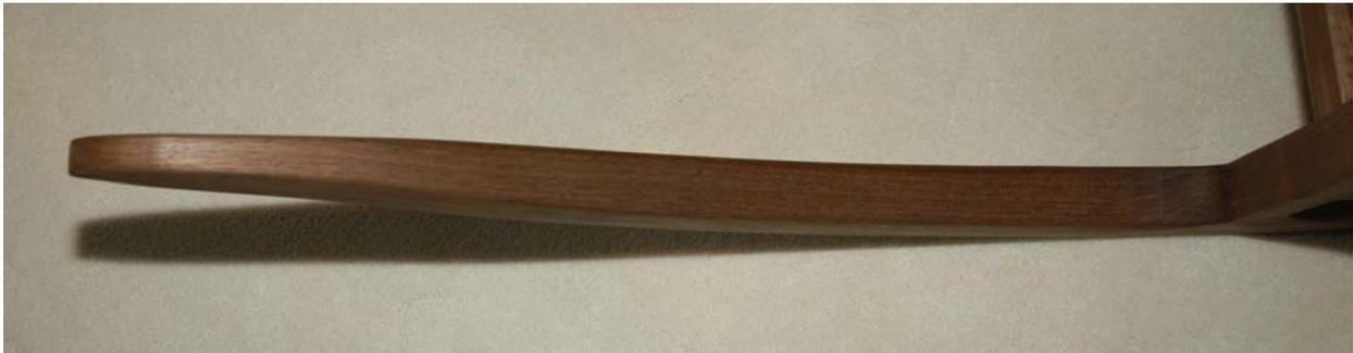
I also did a buildup where the legs will attach to the rockers. I did this by gluing some additional laminates at those locations.
